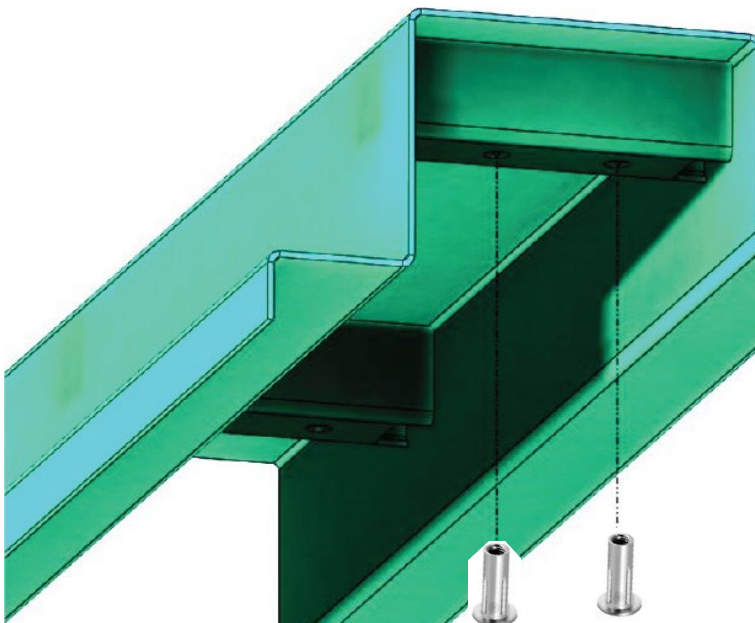
Figure 2: Alternatively use anchor rivet nuts M10
